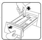
Flush it out under a tap, to remove any traces of accumulated powder.
